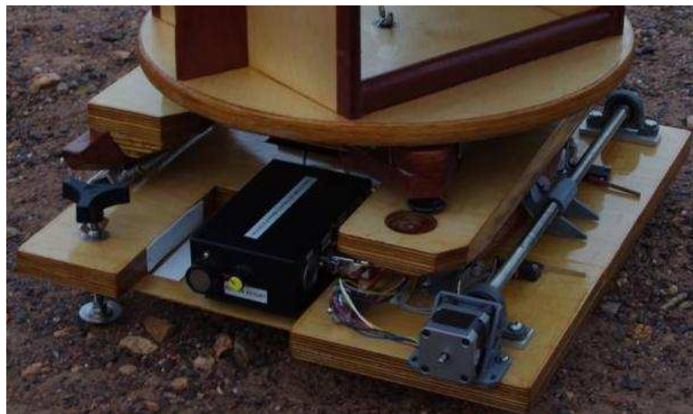
Rod Brackenridge had 2 telescopes set up, the beautifully crafted small Dobsonian at centre has an equatorial tracking platform, also shown in photo below
