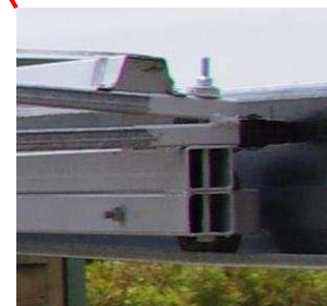
Below - close up view of wheels in "C" beam, small rubber wheel at top helps to keep the roof central & stops any metal rubbing.
